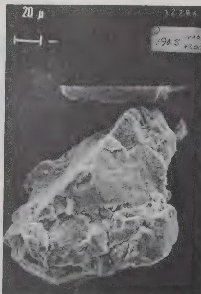
7.6d McMurray Formation Numerous crystal facets. A grain from the Middle Member, an oil-rich zone.
